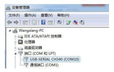
As shown in the figure above, your serial port number is COM10 at this time. Please remember this serial port. You need to fill in the serial port number in the sensor monitoring software.
